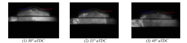
Fig. 7. Occurrence of single flames (surface ignition) – sequence of flame images (side view) 1000 RPM, 100% 2,2,4, trimethylpentane isooctane, A/F = 14.59 - 14.82
