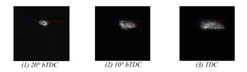
*Fig. 4. Spark-ignition combustion process – sequence of flame images (side view)* 1000 RPM, 100% 2,2,4, trimethylpentane isooctane, A/F =14.59 – 14.82
