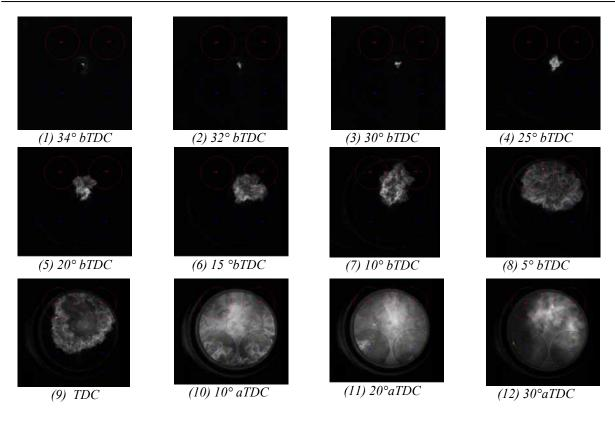
*Fig. 3. Spark-ignition combustion process – sequence of flame images (bottom view)* 1000 RPM, 100% 2,2,4, trimethylpentane isooctane, A/F =14.59 – 14.82
